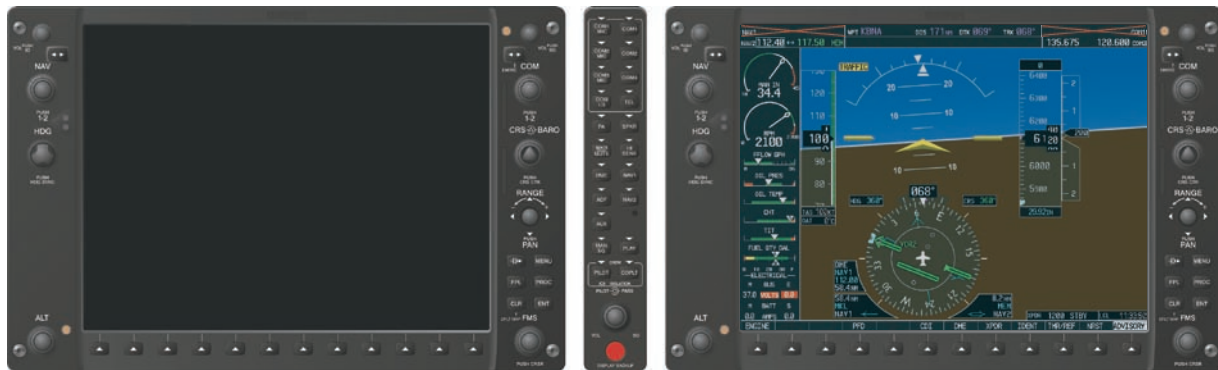
Figure 1-9 Reversionary Mode (Failed PFD)
