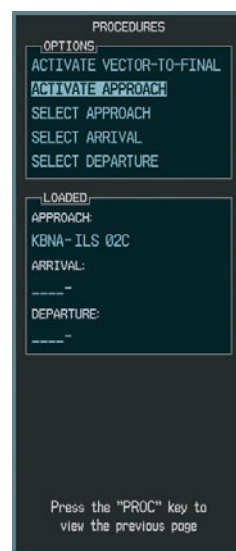
Figure 3-31 Activating an Approach
