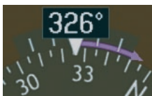
Figure 2-15 Turn Rate Indicator and Trend Vector
