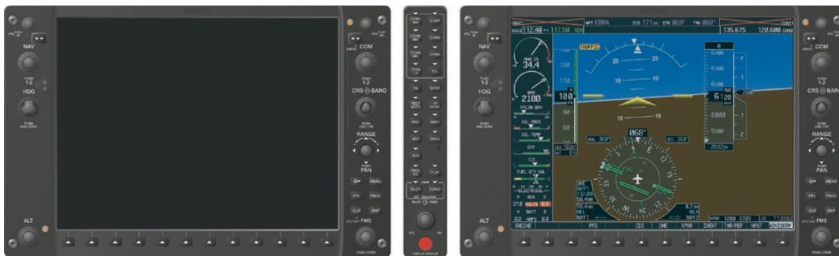
Figure 2.7.2 Reversionary Mode (Failed PFD)
